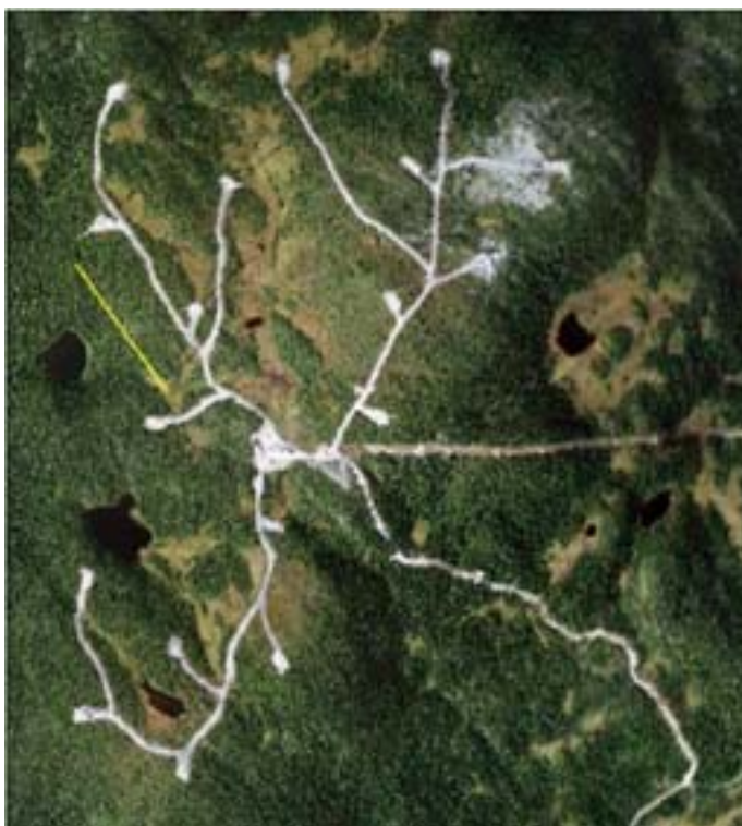
The wind farm at Bliekevare, Västerbotten county, Sweden, where ca 9 km new road has been constructed, and the average width of the road area is 21 m (Rönnqvist 2011). A 500 m line (yellow) is inserted in the picture for scaling. At the time of the image the wind farm is under construction. From Google Earth.
