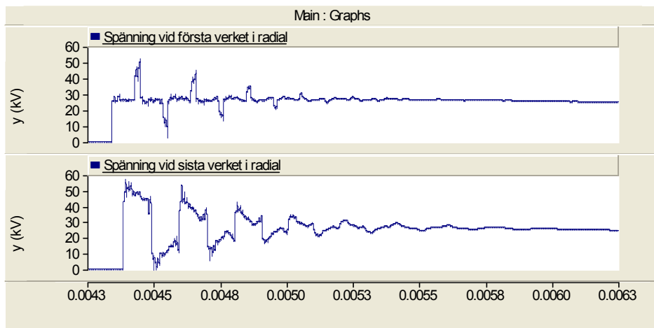
Figure 7. Phase voltage at the first (upper graph) and last (lower graph) turbine in a radial grid when a vacuum breaker is switched during simulation at Kriegers Flak.
