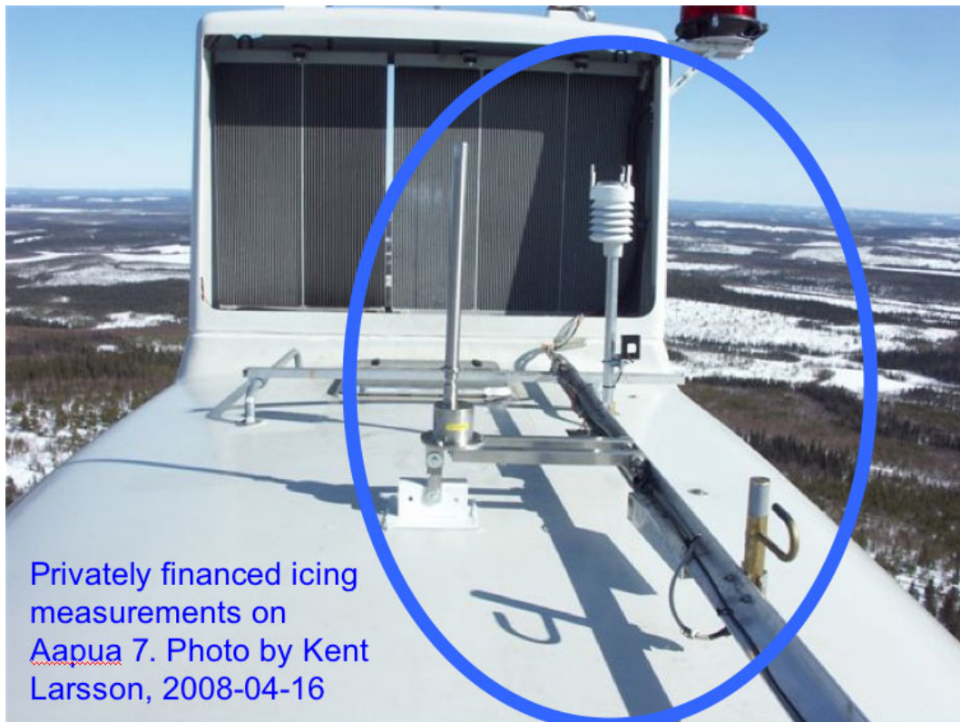
Figure 4: Icing measurement set-up on Aapua 7.
